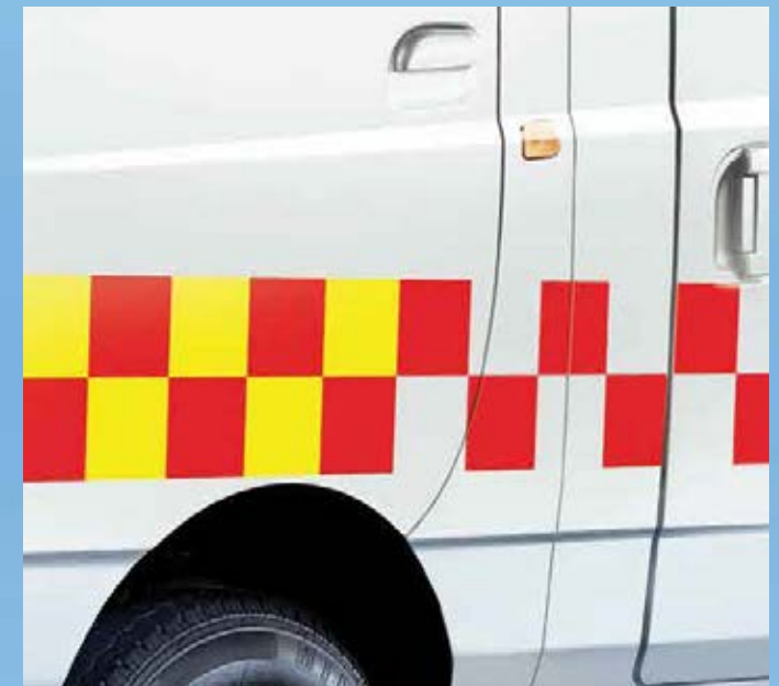
Retro-reflective decals as per AIS 125 norms
